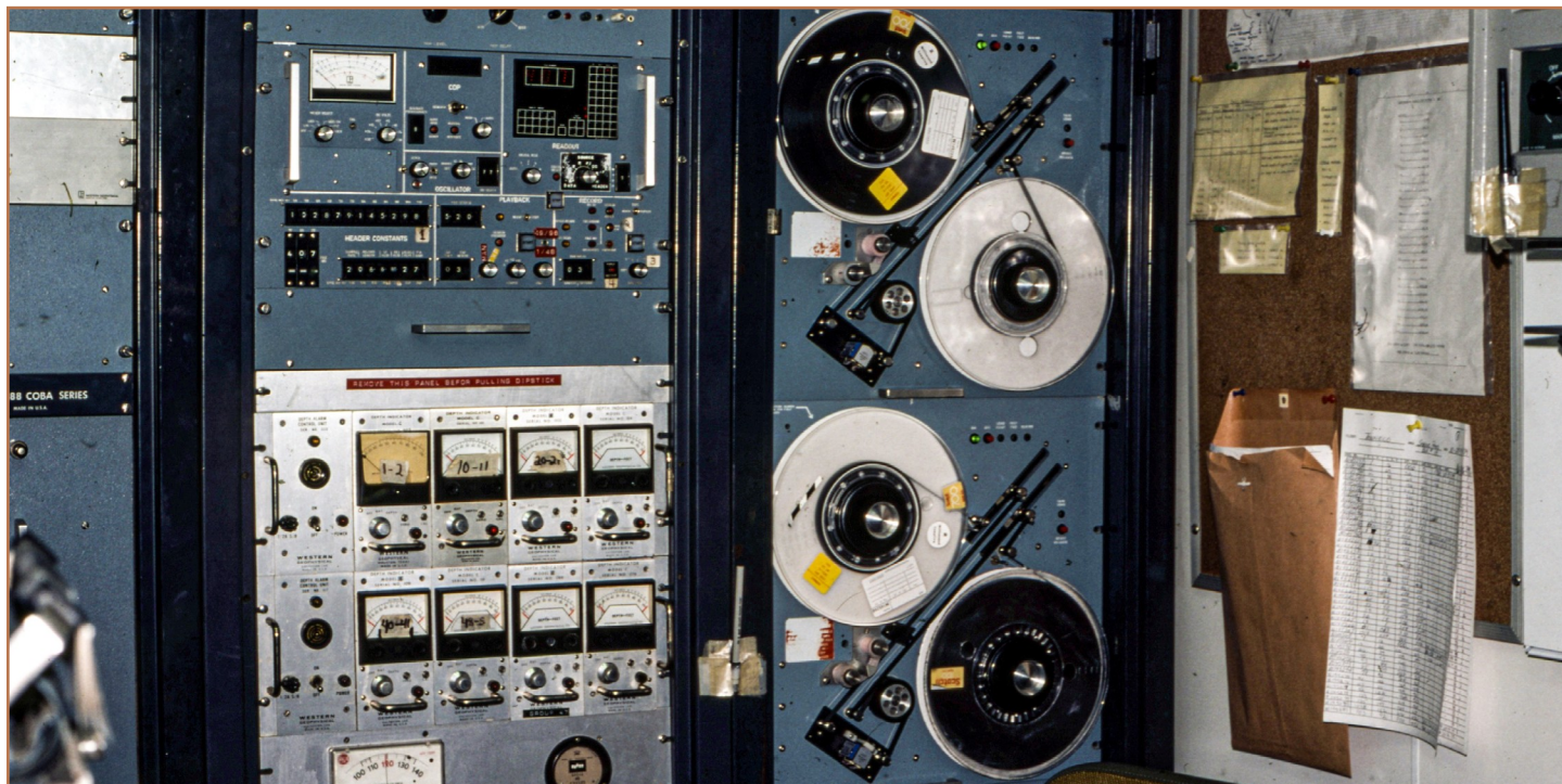
Figure 2: Two banks of the Western Geophysical LRS-888 COBA recording system. The upper left panel contains controls for various recording and playback parameters, including streamer test controls. The lower left panel contains depth gauges for portions of the streamer that have birds (depth control devices). The right bank was our two tape drives loaded with 3M Black Watch 700 tapes. The top drive is almost finished recording; the bottom drive is fresh and will take over when the top drive runs out of tape. On the top of the corkboard, to the right, is a section of shot readout where I labeled the various components of the record. I would post different things on this board, including stack sections that I had interpreted, to teach the crew the science behind the work we were doing. The fathometer is partially visible on the far right.
