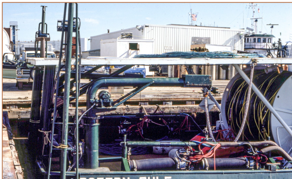
Figure 3: The back deck of the M/V Western Gulf showing the streamer reel and one of the 2-gun Aquapulse arrays. Another gun array is partially visible on the far side of the back deck. Spare streamer sections can be seen on the awning over the back deck. This picture was taken at the Western Geophysical dock on Pelican Island in 1980. On the far-right side of the photo, the superstructure of one of the larger 'Green Meanie' boats can be seen and a second mast behind it.
