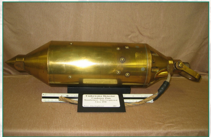
Petty Submersible Refraction Detector from 1929
