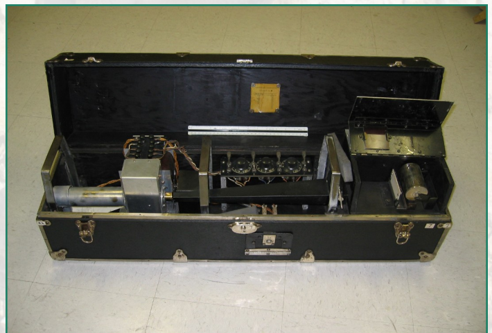
Petty Seismic Refraction Recorder from 1927
