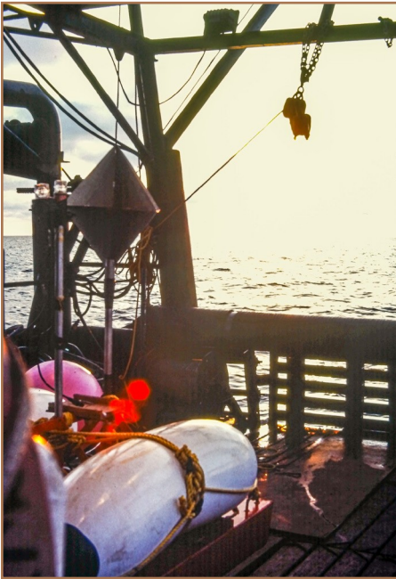
Figure 3: Streamer recovery operations complete! Back deck all tidied up and reroute to the next location. The only thing visible in this picture is the tail buoy with its radar reflector, transmitting antenna and light, and the large sausage buoys that were strapped to the top of the metal frame to (hopefully) keep it upright while being pulled behind the boat.
