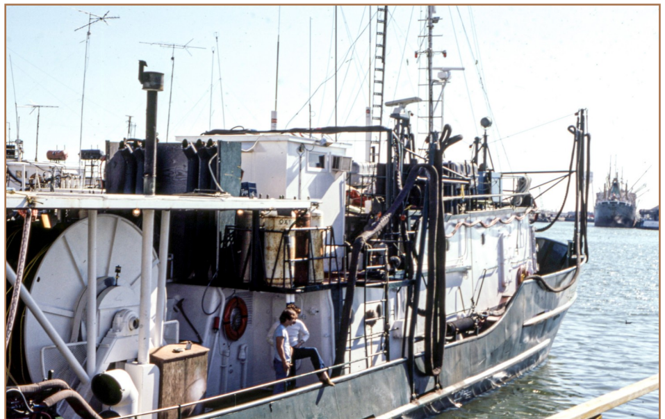
Figure 1: Side shot of the M/V Western Gulf showing the cable reel (left) and the 'shoot shack' above the rear of the boat's upper deck. The 'doghouse' (recording room) is directly beneath the shoot shack. The two gun (seismic source) booms can be seen amidships and on the bow. At the rear of the shoot shack on the starboard (right) side the oxygen tanks can be seen (one labeled with 'oxy'). This was one half of the combustible material for the guns. The other material, propane, was located in similar tanks on the port (left) side of the shoot shack.
