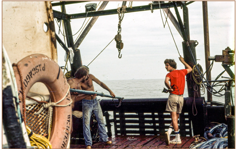
Figure 2: Streamer recovery operations during 'back down and drag' acquisition. In this picture, I'm taking one of the chain strings off of the streamer while another person holds the streamer to keep it from spinning. The person to the right is holding a microphone/speaker that was connected directly to the bridge and which he would use to guide the boat so the streamer kept straight behind the boat as it was going in reverse.
