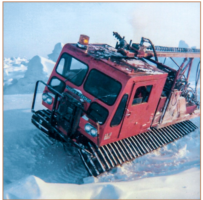
Figure 2: Canadair Flextrac CF 10 tracked drill vehicle. This photo depicts a common occurrence of the track slipping off the wheels. To get it back in place you spread the track with the use of a "Jack All". Once, the jack slipped out of position striking me directly on the knee. Ouch! Fortunately that only happened once.
