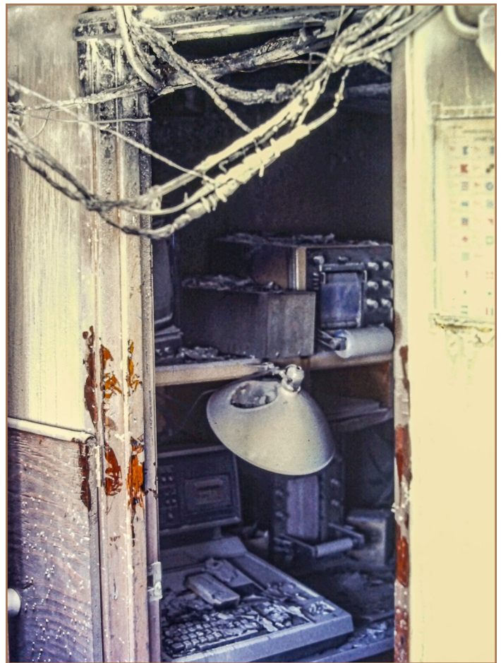
Figure 2: Looking into the nav room which was just opposite of the chart table from Figure 1. As you can see, it was a total loss due to the heat and smoke. The worst damage was along the ceiling which was where flames were spewing out of the air vents.
