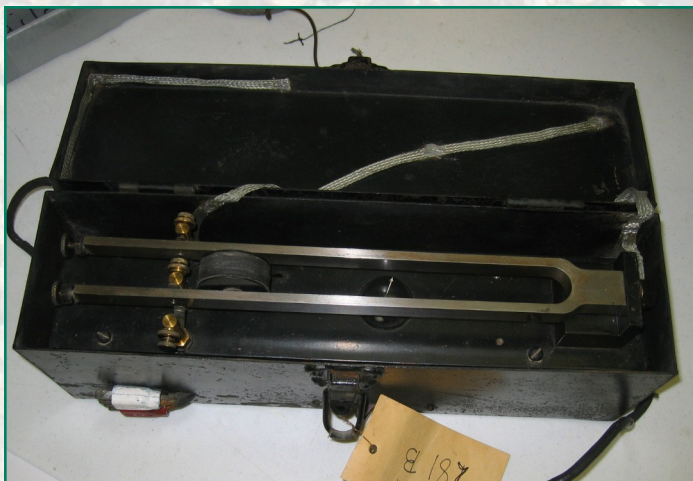
A 50 cycle per second tuning fork
