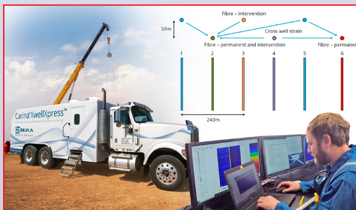
Figure 2. Multiple well monitoring using permanent and intervention engineered sensing cables. Intervention engineered fiber cable provides a new accessible dimension for crosswell monitoring
