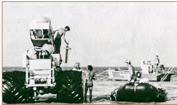
Figure 6: These three pieces of equipment – a rubber Zodiac boat, a jet boat, and a drill buggy – all belong to marine Party 181 and worked together during a land tie at low tide in the Red Sea.
