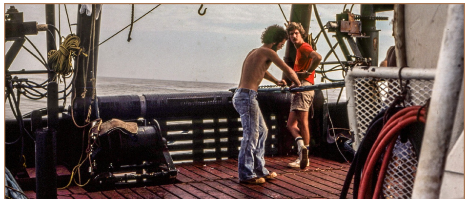
Figure 2: Junior Observer Scott Singleton removing chains from the steamer as it was recovered. These chains were what held the steamer in close proximity to the seasoner for a type of shooting called "back down and drag", which was how data was acquired in shallow water. In the background is Observer Peter Van Borssum making sure the bridge kept the steamer directly behind us as the vessel went in reverse to pick it up. (Photo from Scott Singleton, 1979)
