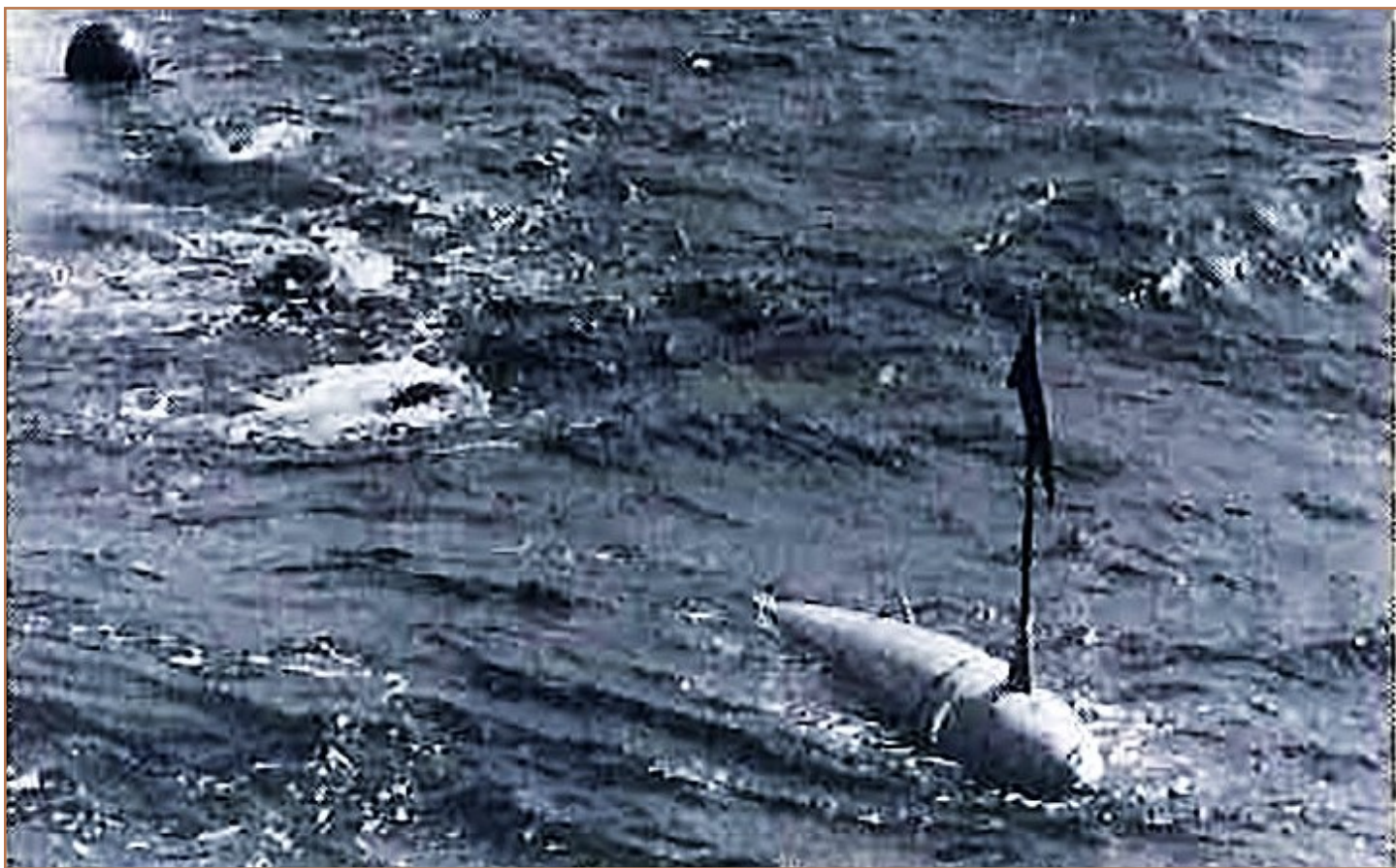
Fig 2: A steel dolphin leads an airgun string. These floats were used to guide the arrays and to provide for their added visibility.
