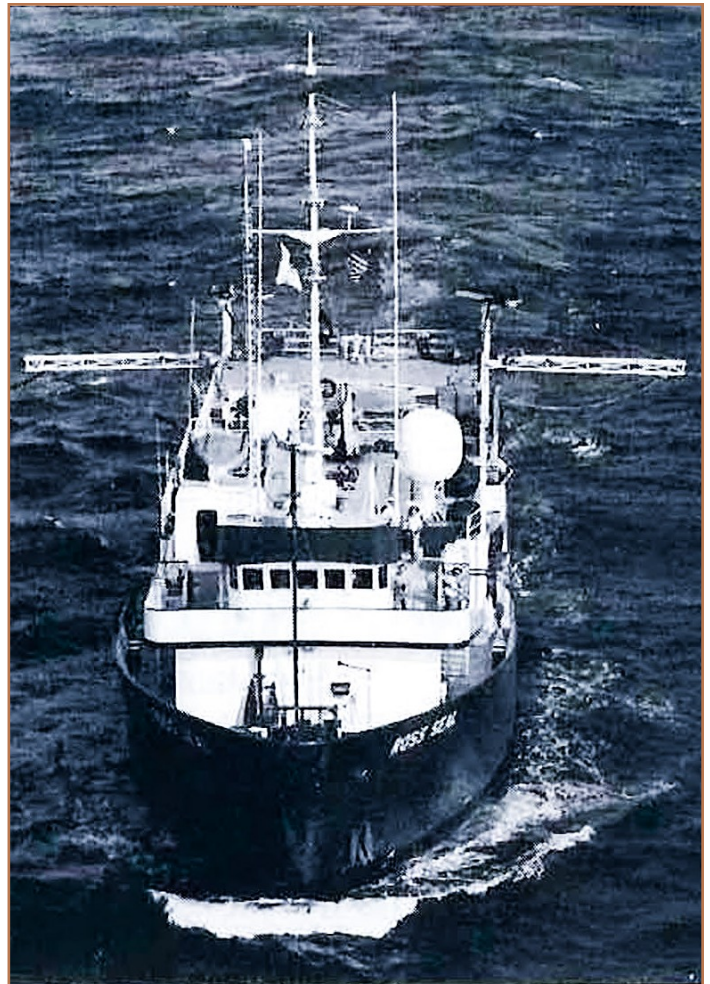
Fig 1: Let wide tow broaden your horizons. The M/V Ross Seal with outriggers on the stern to allow airgun arrays to be towed some distance from each other.
