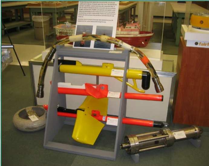
"Birds" for marine seismic cable control
