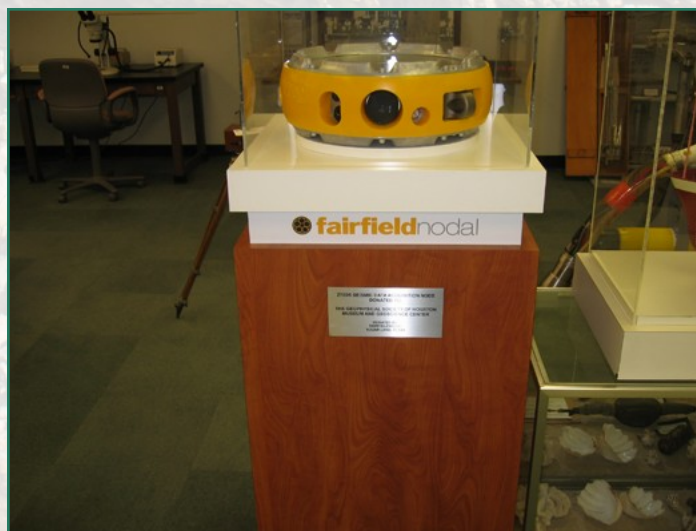
Z node marine seismic acquisition module
