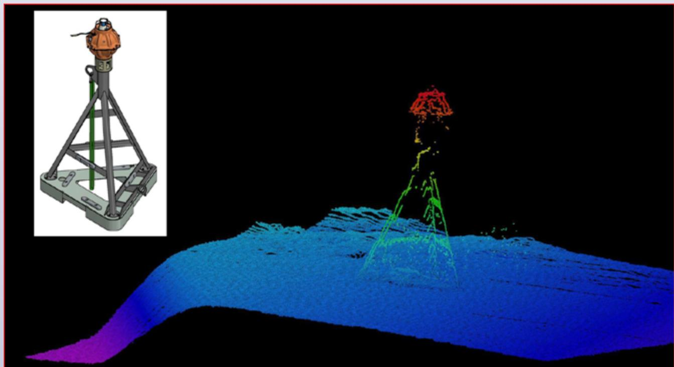
*Figure 7: Laser scan of a 3-m high PMT device compared to a drawing of the instrument (inset)*
