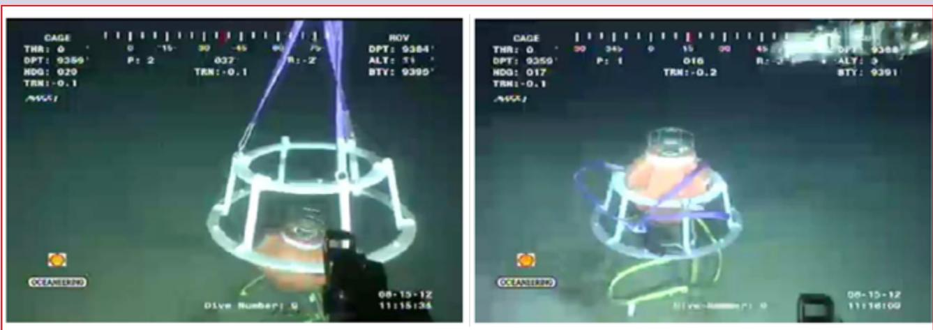
**Figure 3: Weight collar being installed on an PMT device.**
