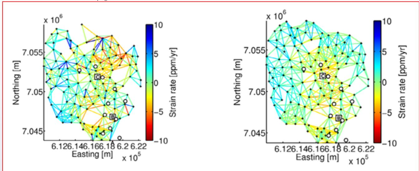
*Figure 6: Measured (left) vs. modeled (right) strain rates at Ormen Lange. Each line represents a ranging arc between two PMT's. Green denotes no horizontal displacement, blue shows extension and red shows contraction.*
