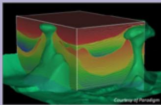
Seismic image with velocity model overlaid and interpreted salt bodies (Courtesy of Paradigm).
