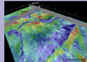
FWI velocity model overlaid on the depth seismic image (Courtesy of PGS).
