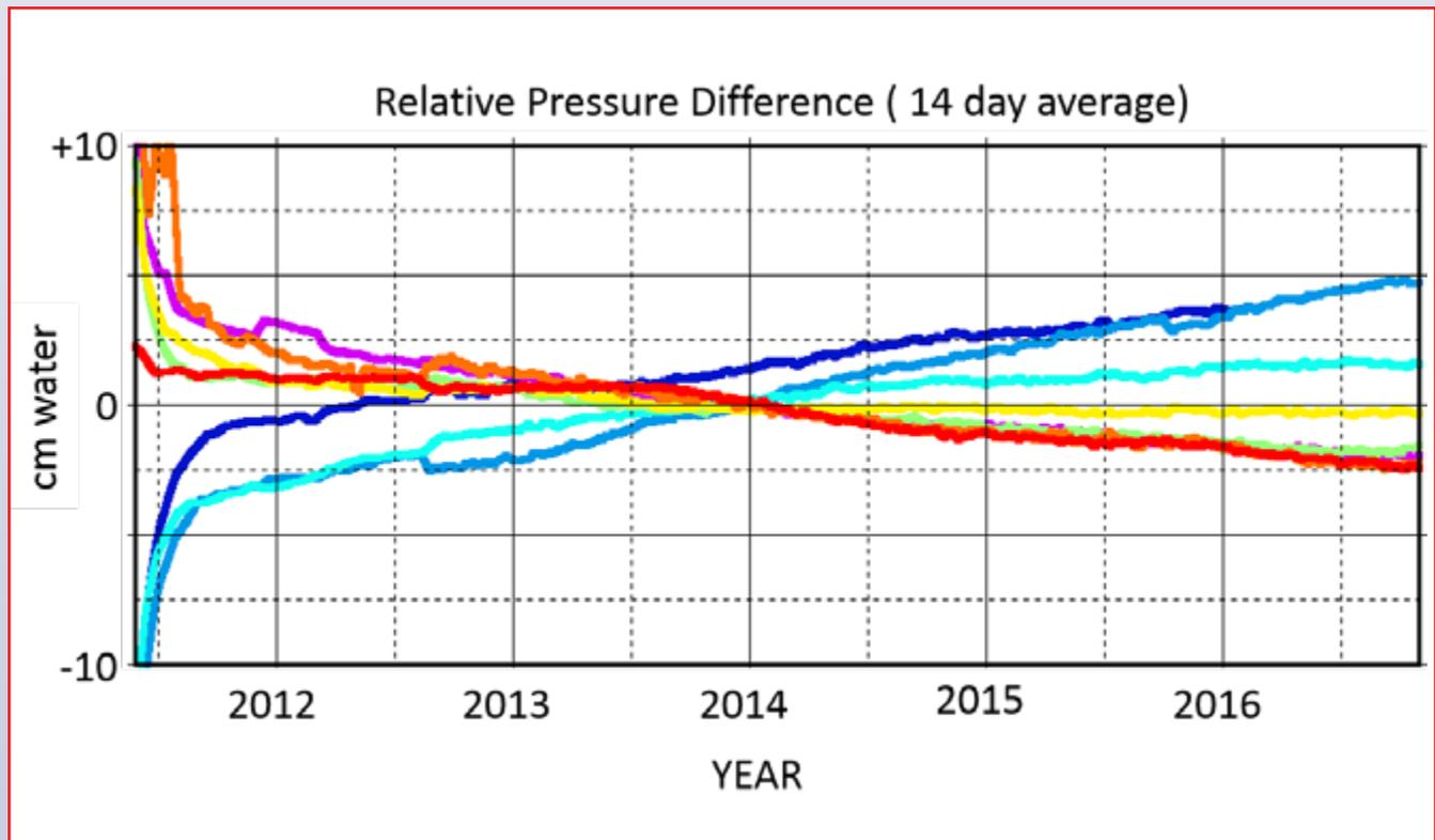
Figure 2: Relative pressure differences (displayed in cm of water) between several pressure sensors deployed for more than 5 years in the GoM.
