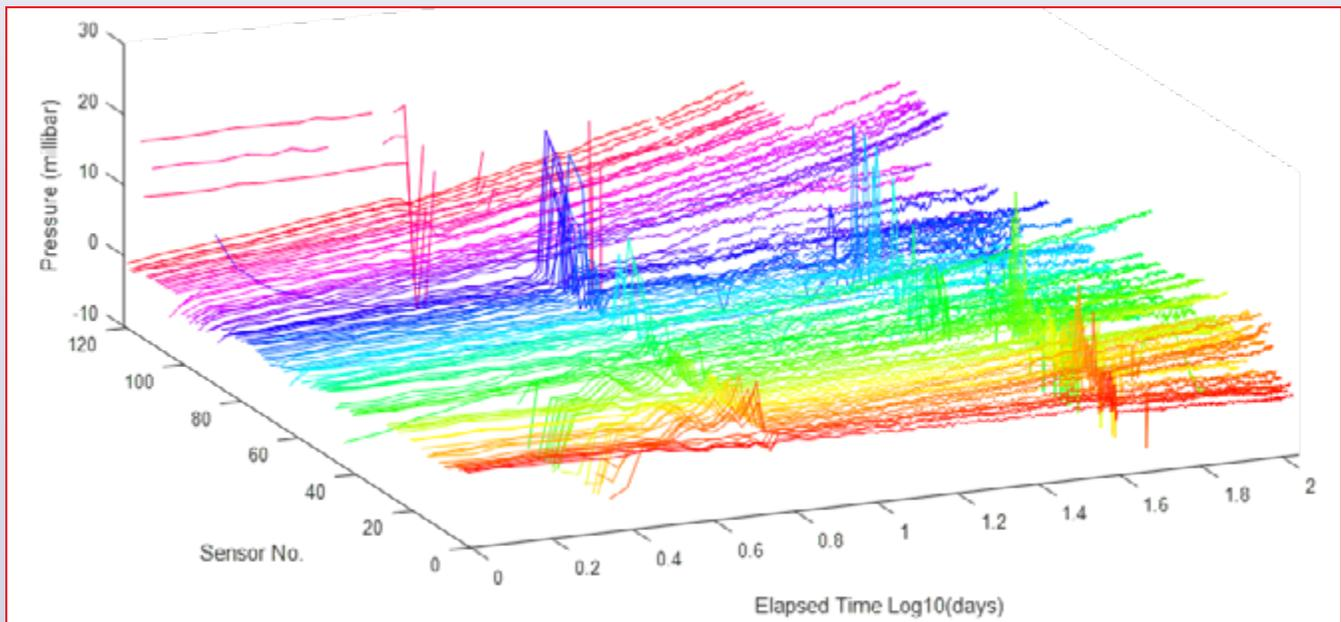
Figure 5: 120 pressure sensors held at the same temperature and pressure for months enabling drift characteristics to be determined and badly behaving sensors to be detected.
