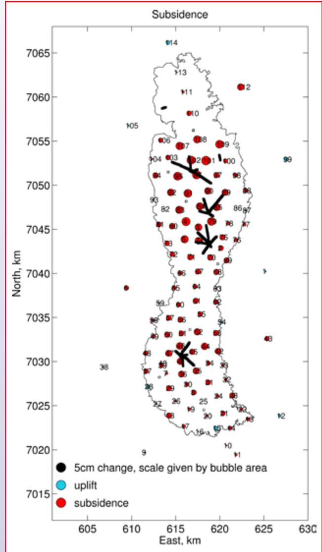
Figure 1: Subsidence observations in the deepwater Ormen Lange field using the method of Eiken et al (2000; 2008).
