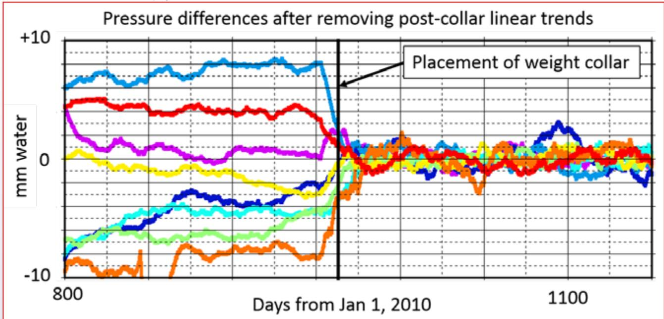
Figure 4: Sudden change in pressures that occurred when weight collars were placed on the PMT instruments.
