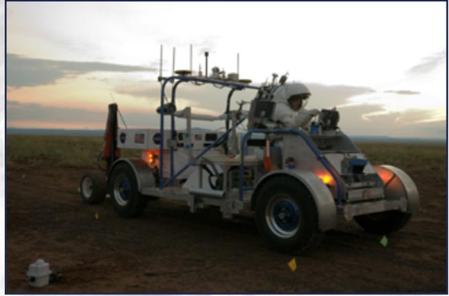
Testing of an elastic weight drop source on a seismic reflection line at Meteor Crater, AZ using a wireless receiver system integrated with a surface exploration vehicle in a next generation space suit.
